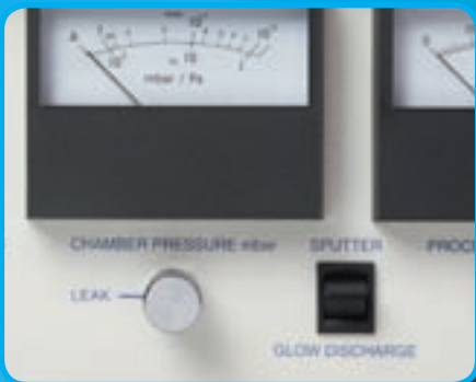
Switch to change between sputtering and glow discharge modes
