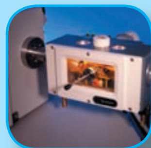
Cryo preparation chamber
