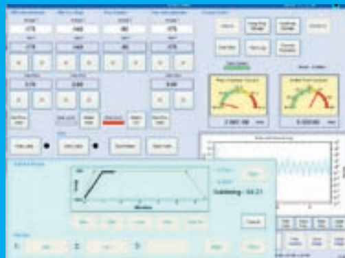
Sublimation parameters for temperature and time can be pre-set and stored
